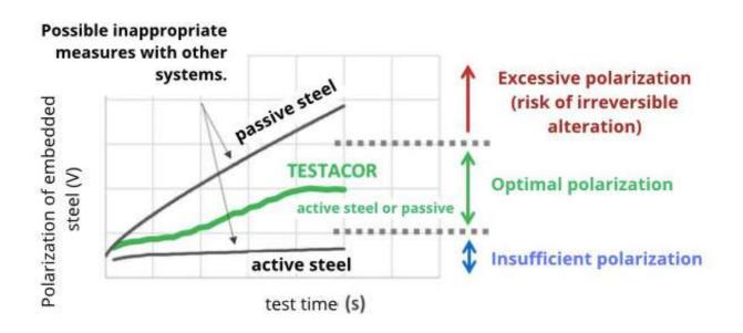
Fig.1 Optimal Polarization Achieved with Testacor During the Test Compared to Possible Undesirable Situations with Other Systems
